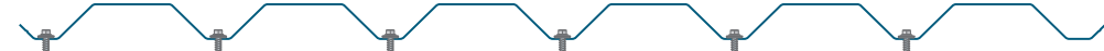
Figure 01: Fixing positions for roof and wall profiles - to achieve optimum sealant compression
